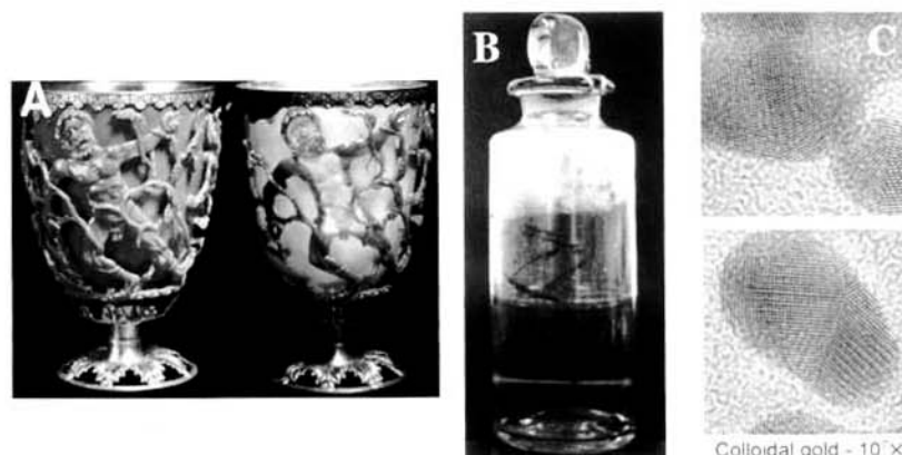
Figure 1.2. (A) Lycurgus cup showing two different colors in reflected light (green) and transmitted light (red) ( adapted from the web site of The British Museum ). (B) Faraday's colloidal suspension of gold with a clearly visible red laser beam and (C) the high resolution transmission electron microscope images of individual colloidal gold particles ( adapted from reference 24 ).
