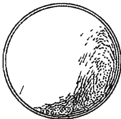
Figure 4.15 (a): Vector plot of centrifuging motion after 1 rotation
