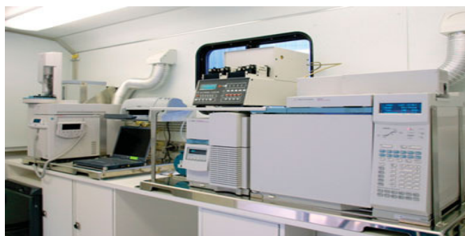
Photograph 1a Mobile lab donated by Agilent Technologies to NYPD. b) Interior of mobile lab showing Agilent 6890 GC with mass-selective detector [Smith, 2002].
