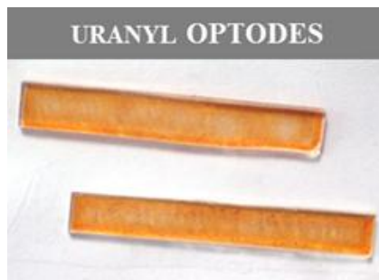
Figure 5.5 Fabricated IPI optodes after proper drying
