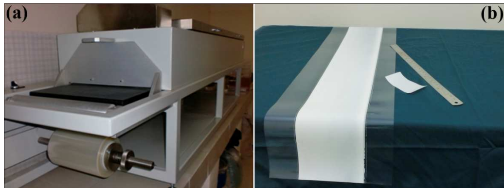
Figure 2.7 Photographs of (a) tape casting machine and (b) cast LTCC tape.
