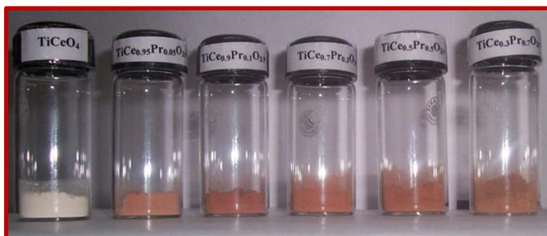
**Fig. 3.4.** Photograph of  $\text{TiCe}_{1-x}\text{Pr}_x\text{O}_4$  ( $x= 0, 0.05, 0.1, 0.3, 0.5$  and  $0.7$ ) pigments.
