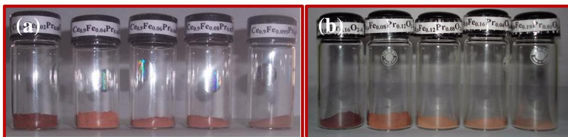
**Fig. 2.14.** Photographs of (a) Ce<sub>0.9</sub>Fe<sub>x</sub>Pr<sub>0.1-x</sub>O<sub>2-δ</sub> ( $x = 0.02, 0.04, 0.06, 0.08$  and  $0.095$ ) and (b) Ce<sub>0.8</sub>Fe<sub>x</sub>Pr<sub>0.2-x</sub>O<sub>2-δ</sub> ( $x = 0.04, 0.08, 0.12, 0.16$  and  $0.19$ ) pigments.
