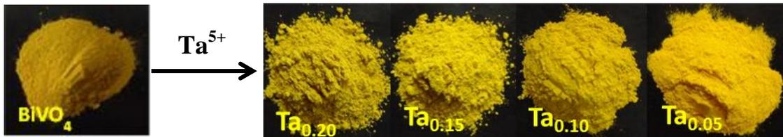
Fig. 5.9. Photograph of  $\text{BiV}_{1-x}\text{Ta}_x\text{O}_4$  ( $x = 0, 0.05, 0.10, 0.15$  and  $0.2$ ) pigments.
