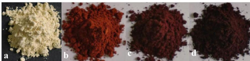
**Fig. 1.9.** Photographs of  $\text{Y}_2\text{Ce}_{2-x}\text{Pr}_x\text{O}_7$ : (a)  $x = 0$  (b)  $x = 0.1$  (c)  $x = 0.3$  and (d)  $x = 0.5$  pigments.
