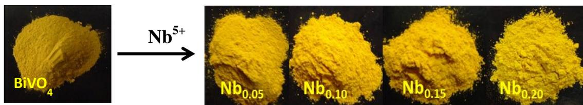
**Fig. 5.7.** Photograph of  $\text{BiV}_{1-x}\text{Nb}_x\text{O}_4$  ( $x = 0, 0.05, 0.10, 0.15$  and  $0.2$ ) pigments.
