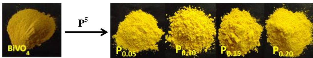
Fig. 5.11. Photograph of  $\text{BiV}_{1-x}\text{P}_x\text{O}_4$  ( $x = 0, 0.05, 0.10, 0.15$  and  $0.20$ ) pigments.
