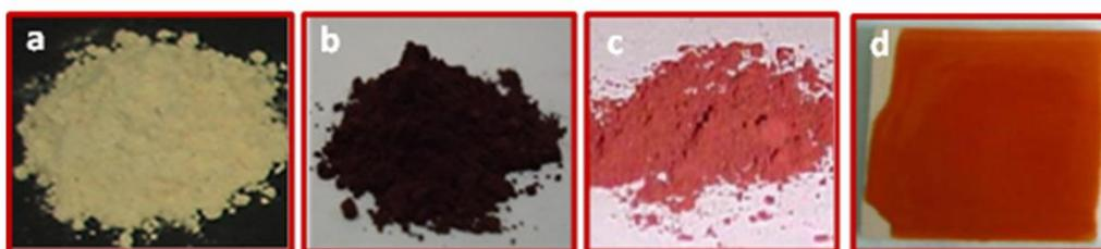
**Fig. 1.8.** Cerium based red pigments (a)  $\text{CeO}_2$ , (b)  $\text{Ce}_{1-x}\text{Pr}_x\text{O}_2$ , (c) (55% $\text{Fe}_2\text{O}_3$ -40% $\text{CeO}_2$ ):5%Pr and (d)  $\text{Ce}_{0.8}\text{Tb}_{0.2}\text{O}_{2-y}$ .
