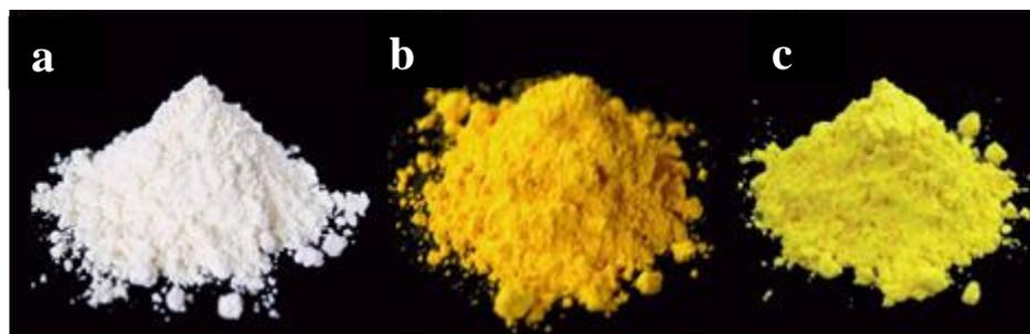
**Fig. 1.13.** Photographs of (a)  $\text{Ce}_{0.43}\text{Zr}_{0.37}\text{La}_{0.20}\text{O}_{1.9}$ , (b)  $\text{Ce}_{0.43}\text{Zr}_{0.37}\text{Bi}_{0.20}\text{O}_{1.9}$  and (c) praseodymium yellow.
