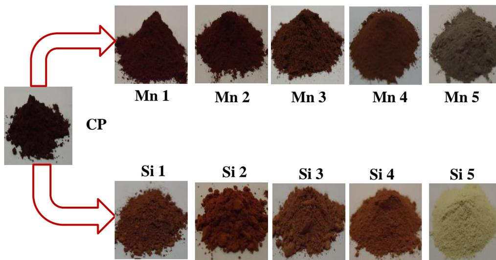
**Fig. 2.18.** Photographs of Ce<sub>0.95</sub>M<sub>x</sub>Pr<sub>0.05-x</sub>O<sub>2</sub> (M=Mn<sup>4+</sup>/Si<sup>4+</sup>; *x* = 0, 0.01, 0.02, 0.03, 0.04 and 0.05) pigments.
