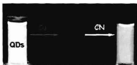
Figure 4.3. QD based luminescence 'turn ON' sensor. The Cu(II) on QD surface quenches QD luminescence, which is restored in the presence of CN - ( adapted from reference 4 ).
