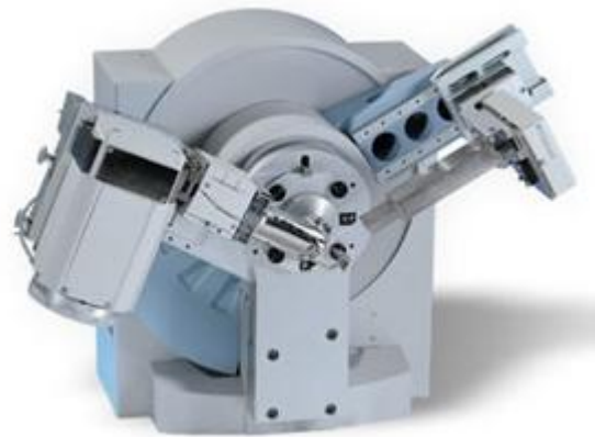
Fig. 2.4 Reflection and transmission geometry in X ray diffraction and Goniometer in PANalytical X'pert PRO X ray diffractometer.
