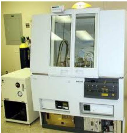
Fig. 2.4 Reflection and transmission geometry in X ray diffraction and Goniometer in PANalytical X'pert PRO X ray diffractometer.
