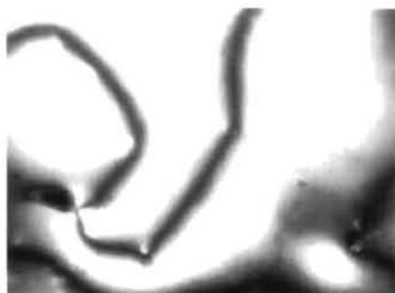
**Figure 3.4.** Polarized optical micrograph (400x) showing Schlieren texture of a nematic phase obtained for **BC1** at 194.7 °C.
