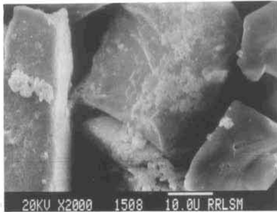
Fig.2.15. Scanning electron micrographs of magnetic fraction after removing the adhered clay fraction in 5M NaOH solution. c&d-spongy appearance of muscovite indicating initial stages of alteration (sample KK); e-clusters of goethite in sample KK
