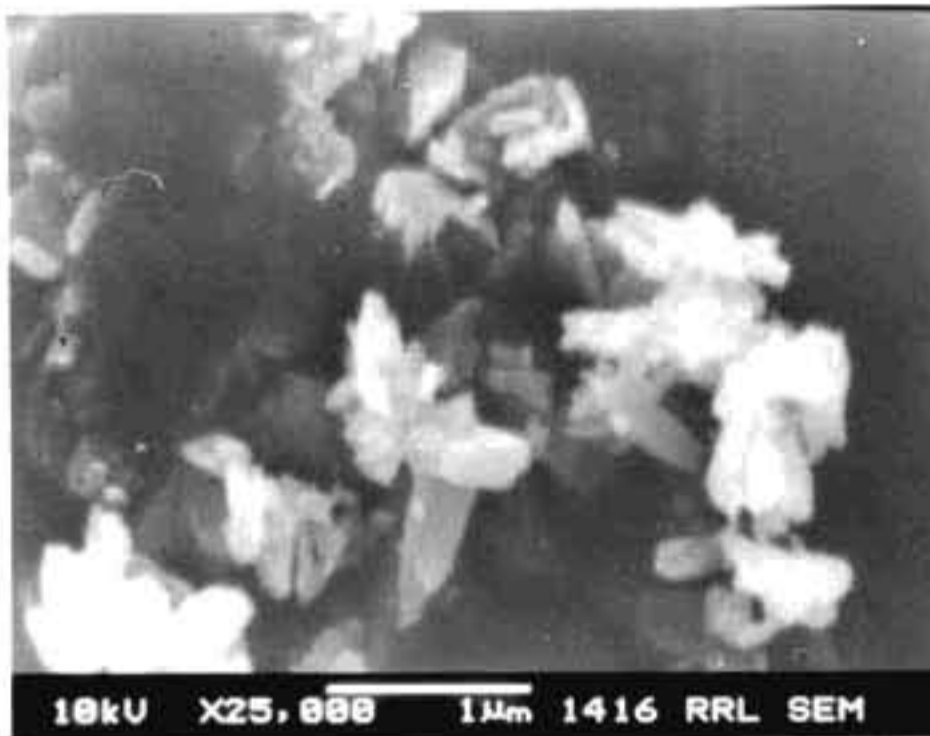
Fig.5.5. Natural goethite in sample TK after removing the clay fraction in 5M NaOH solution
