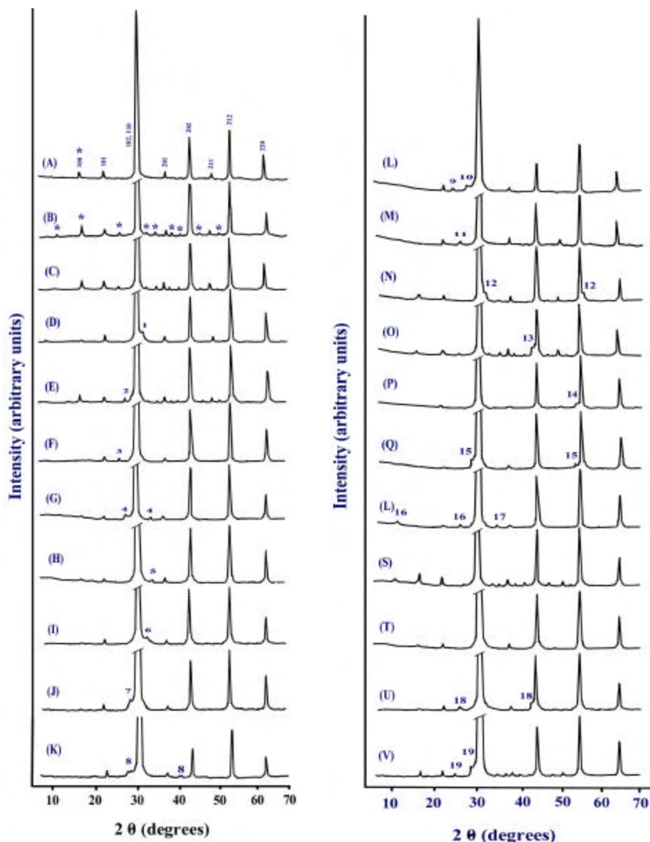
Fig. 4. 2 Powder Diffraction pattern of BMT doped with 5 mole % of the additives: (A) Pure and Unannealed, (B) Pure and Annealed, (C) BMT doped with \text{MnCO}_3 , (D) \text{NiO} , (E) \text{ZnO} , (F) \text{Co}_3\text{O}_4 , (G) \text{Al}_2\text{O}_3 , (I) \text{Fe}_2\text{O}_3 , (J) \text{In}_2\text{O}_3 , (K) \text{Nd}_2\text{O}_3 , (L) \text{Bi}_2\text{O}_3 , (M) \text{CeO}_2 , (N) \text{TiO}_2 , (O) \text{SnO}_2 , (P) \text{ZrO}_2 , (Q) \text{HfO}_2 , (R) \text{V}_2\text{O}_5 , (S) \text{Sb}_2\text{O}_3 , (T) \text{Nb}_2\text{O}_5 , (U) \text{WO}_3 , (V) \text{MoO}_3 . 1 stands for \text{Ba}_3\text{NiTa}_2\text{O}_9 , 2 for \text{Ba}_4\text{Ta}_2\text{O}_9 , 3 for \text{BaCoO}_{2.93} , 4 for \text{Ba}_{10}\text{Al}_2\text{O}_{13} , 5 for \text{BaGa}_{12}\text{O}_{19} , 6 for \text{Fe}_4\text{Ta}_2\text{O}_9 , 7 for \text{InTaO}_4 , 8 for \text{Nd}_2\text{O}_3 , 9 for \text{Bi}_2\text{O}_3 , 10 for \text{BaBiO}_3 , 11 for \text{BaCeO}_3 , 12 for \text{BaTiO}_3 , 13 for \text{BaSnO}_3 , 14 for \text{Ba}_2\text{HfO}_4 , 15 for \text{BaZrO}_3 , 16 for \text{BaV}_3\text{O}_8 , 17 for \text{VTaO}_4 , 18 for \text{BaWO}_4 , 19 for \text{BaMoO}_4 . * represent superstructural reflections
