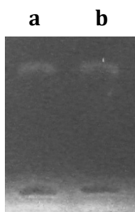
Figure 4.17. Recognition of plasmid PUC18 DNA by the cyclophane 2 after gel electrophoresis through excimer emission. Lanes: (a) 0.05 and (b) 0.1 \mu\text{g}/\mu\text{L} of DNA.
