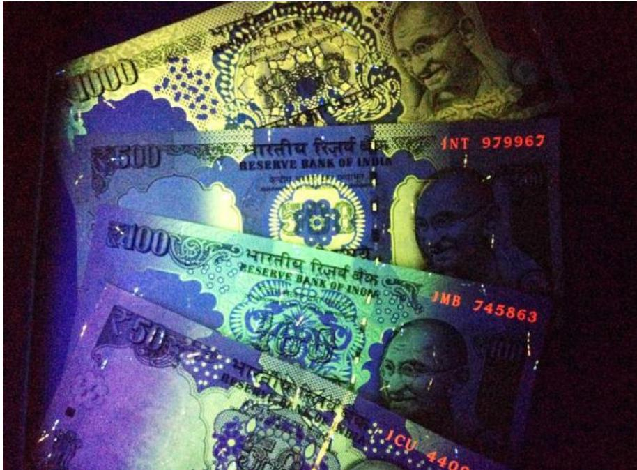
The fluorescent material in a currency note is seen under ultraviolet light.
