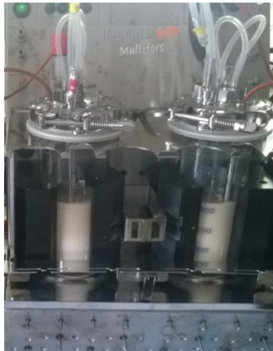
Fig. 4.7. Batch fermentation for folate production in parallel fermenter
