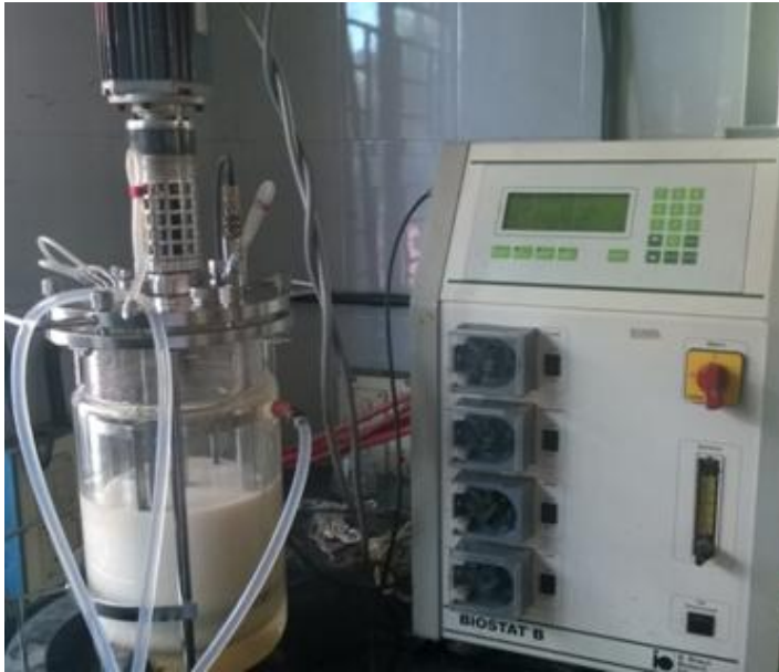
Fig. 4.9. Skim milk fermentation for folate production in 5 L fermenter
