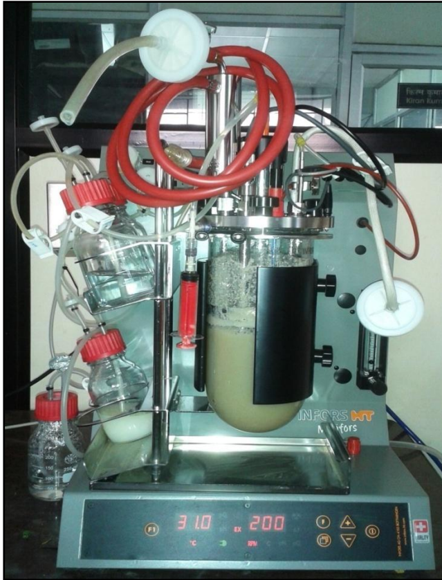
Fig. 2.20. Batch fermentor setup (1L) for chitinase production.
