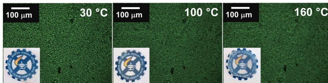
**Figure 2.11.** POM images of PLLA films crystallized in acetone/water mixture measured at (a) 30 °C, (b) 100 °C, and (c) 160 °C. Photographs showing the transparency of PLLA films at different temperatures are shown in the inset.
