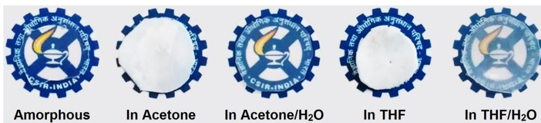
**Figure 2.9.** Photographs showing the transparency of PLLA films crystallized in various solvents. For the purpose of comparison, photograph of amorphous PLLA is also shown.
