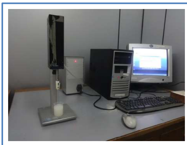
Figure 3.1: Dip-coating set-up used for coating in this study
