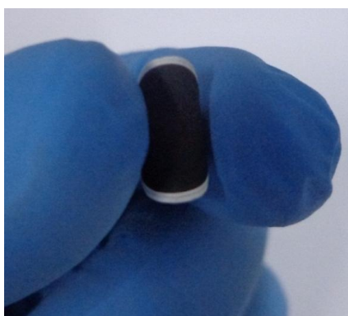
Figure 3.1.10 Photograph of flexible MAXene film prepared by deposition on Nylon 6,6 membrane.
