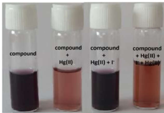
Figure 4.10. Photograph of naked eye detection of \text{Hg}^{2+} with QHQC and its reversibility with iodide solution
