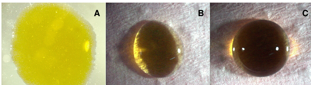
Fig. 4.2.17. Stereomicrographs of water drops on glass slides coated with different VTMS/Si molar ratio A) Uncoated B) 1 C) 2.5
