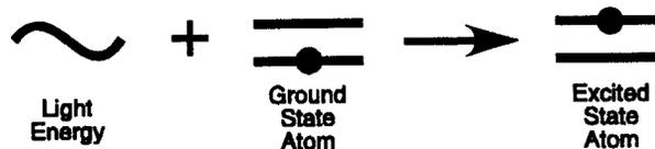
Fig. 2.4A Atomic Absorption Process
