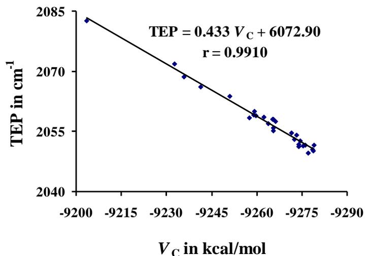
**Figure 2.16** Correlation between MESP at the N-heterocyclic carbene carbon nucleus and TEP.
