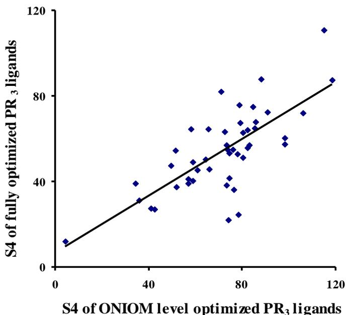
**Figure 2.10** Correlation between the S4 values of fully optimized and ONIOM level optimized PR<sub>3</sub> ligands.
