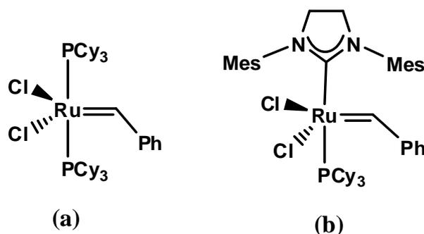
**Figure 4.1** (a) First generation catalyst (b) second generation catalyst.
