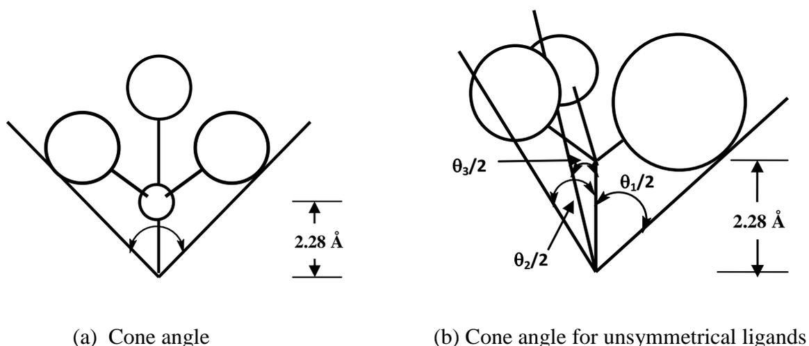
**Figure 2.1** Representation of cone angle
