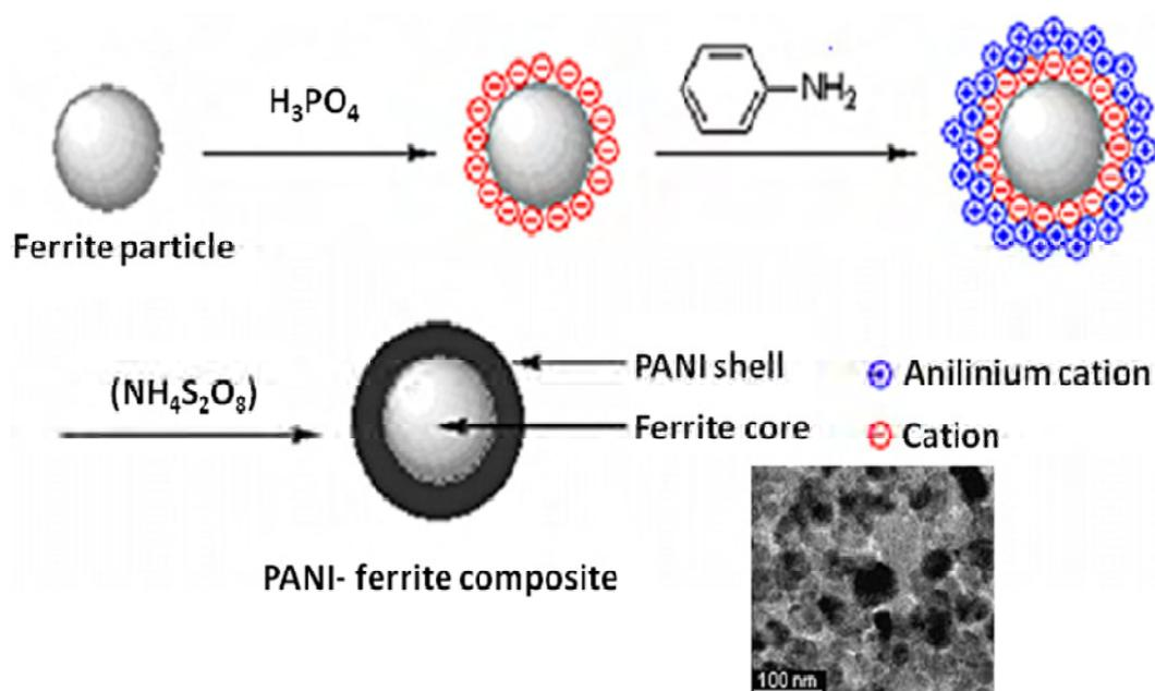
**Figure 1.20.** Polymerization procedure for PANI/  $\text{Zn}_{0.6}\text{Cu}_{0.4}\text{Cr}_{0.5}\text{Fe}_{1.5-x}\text{La}_x\text{O}_4$  composites (inset showing the TEM image of core shell PANI composite)
