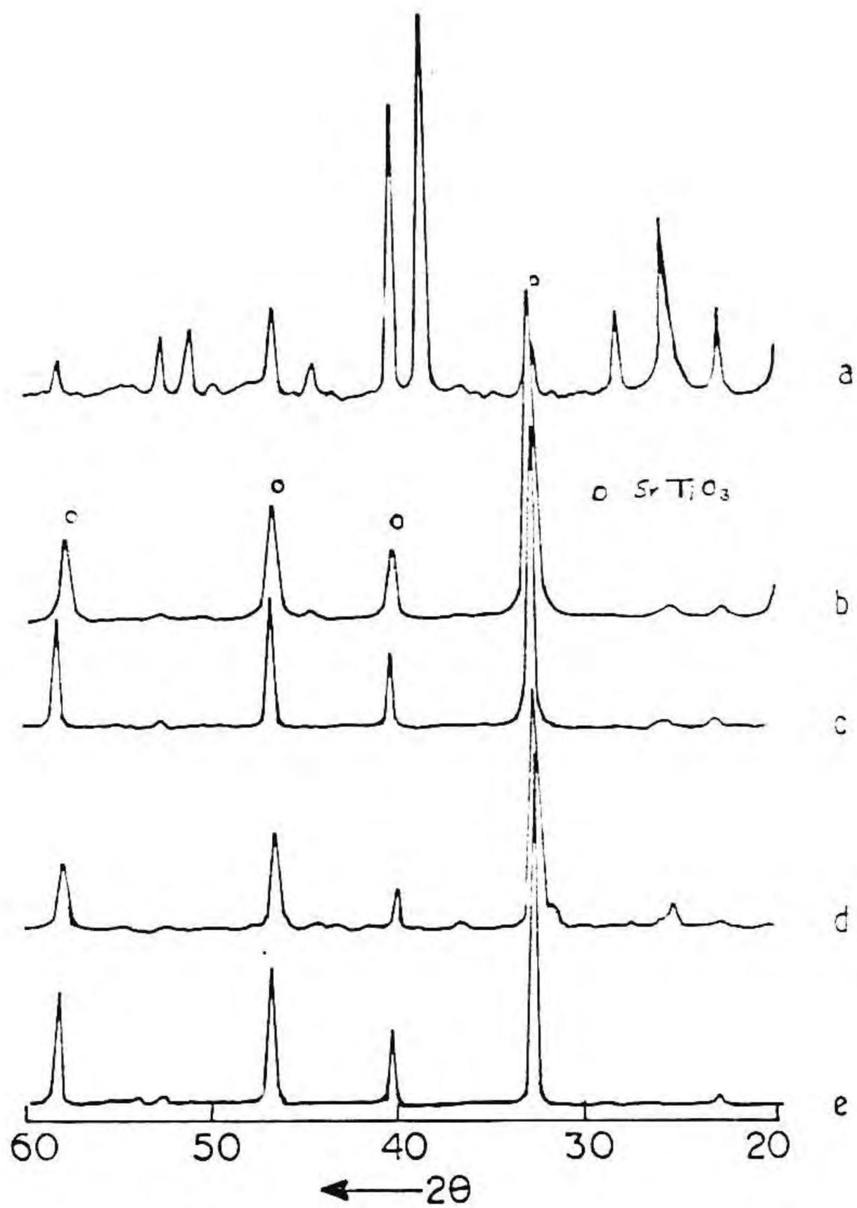
Fig. VIII.3 XRD patterns of the gel sprayed powder heated to different temperatures (a) as sprayed, (b) 650°C, (c) 800°C, (d) 800°C (solid state mixing route) and (e) 1400°C
