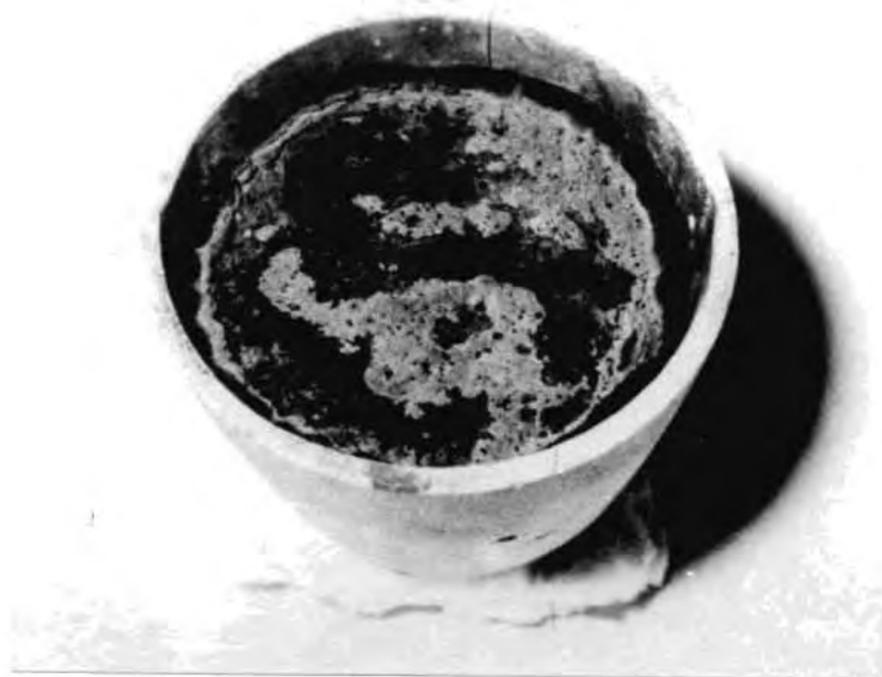
Fig. V.2(b) Precursor powder inside the crucible
