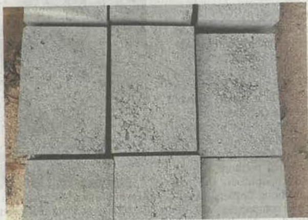
Samples of the brick made from silica sand by Autokast Ltd.
