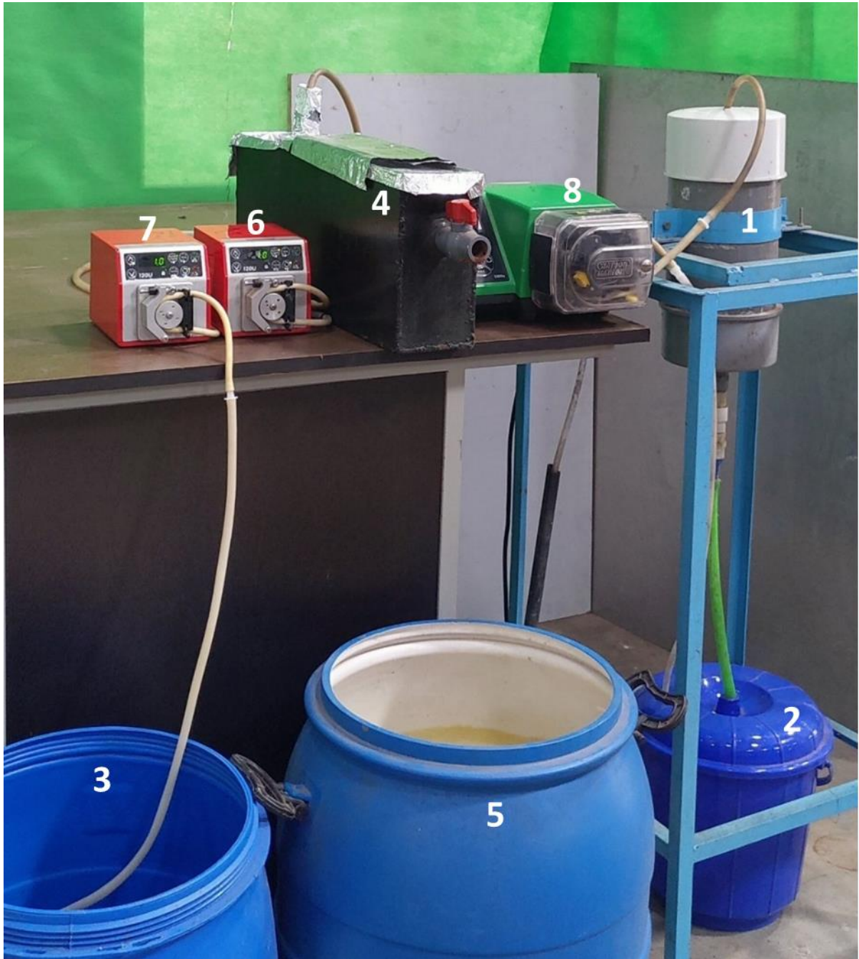
Figure 6.6. Photograph of the combined Anaerobic Leach Bed and Bio-barrier unit used in this study (1 - Anaerobic Leach Bed unit, 2 – Crude leachate collection tank, 3 - Perchlorate feed tank, 4 - Anaerobic Bio-barrier Unit, 5 - Treated water collection tank, 6,7,8 - Peristaltic pumps).
