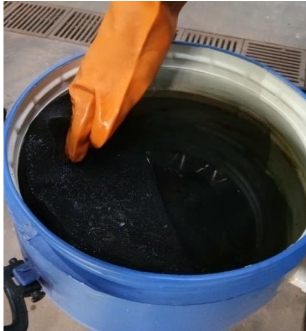
Figure 4.3a. Anaerobic Fixed Film Bioreactor inside showing charcoal filter bed
