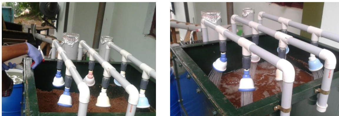
Figure 5.5. Photograph of the overhead shower taps for spraying wash water for soil washing (Left) experiment. The figure also shows the water column logged with water (Right)
