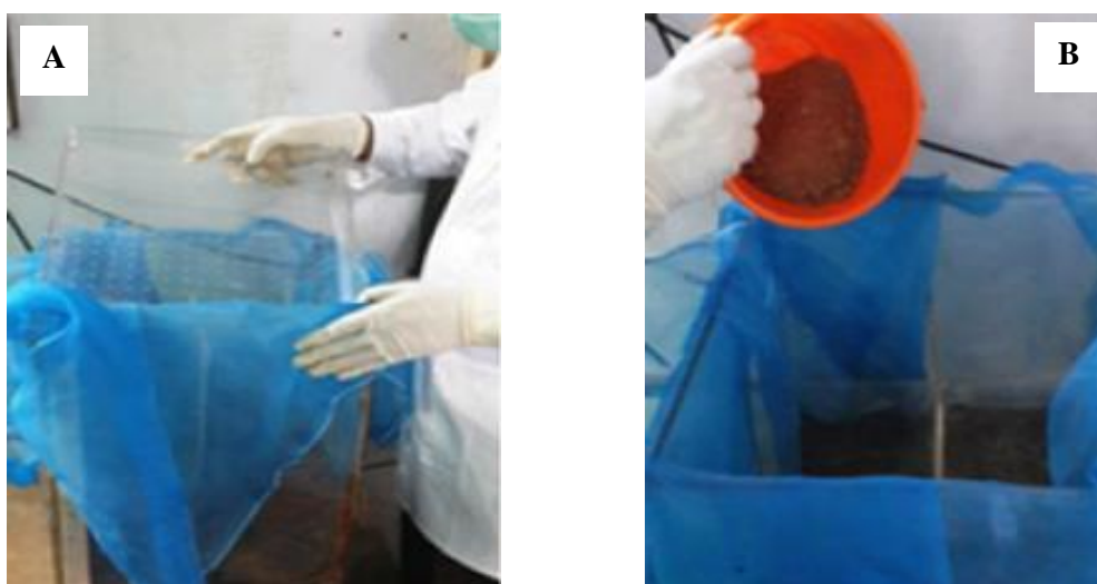
Figure 5.1. Photographs of the box type unit (A) and filling up of the unit with perchlorate spiked soil for washing experiments (B).
