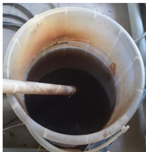
Figure 6.3. Photograph of the organic rich leachate obtained from the anaerobic digestion of the vegetable waste
