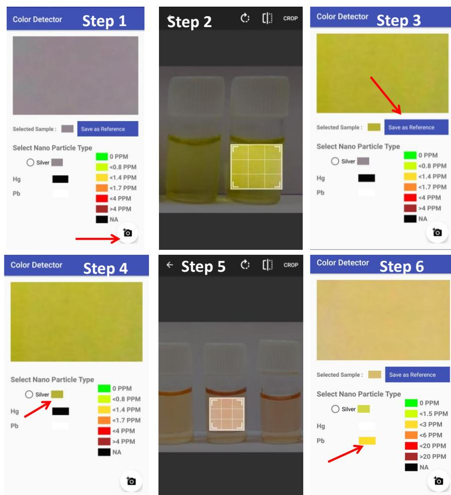
**Figure 6.22.** Developed android application screen (i) step 1: loading the reference sample (pure AgNP) data, (ii) step 2: select the ROI from the reference sample's photograph, (iii) step 3: saving the reference sample image into the database, (iv) step 4: updated the reference sample details and load a new sample, (v) step 5: select the ROI, and (vi) step 6: determined and quantified the metal ion present in the sample as lead and quantified as < 3 ppm.
