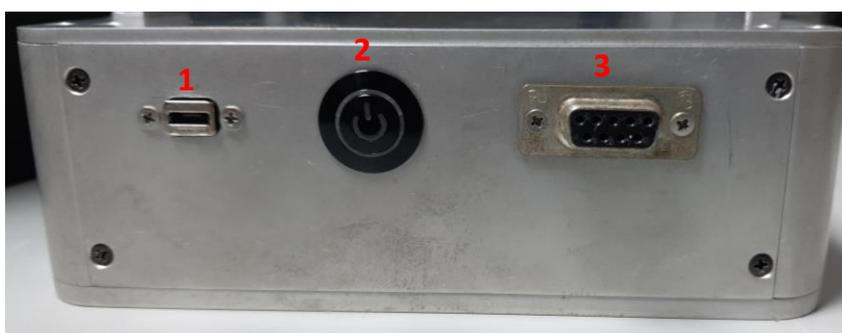
**Figure 3.8.** Photographs showing the interfaces on the sidewall of the chassis, marked as 1. powering port, 2. switch for laser control, and 3. RS232 port to communicate with the tablet PC.
