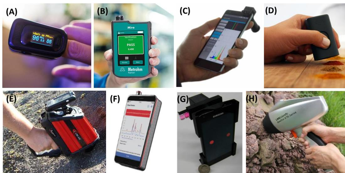
**Figure 1.1.** Photographs illustrating examples for different portable spectroscopic devices for onsite analysis (A) pulse oximeter, (B) handheld Raman spectrometer from Metrohm, (C) GoSpectro handheld spectrometer from GoyaLab, (D) Scio pocket-size NIR spectrometer, (E) A2 Technologies's FTIR spectrometer for soil analysis, (F) Cloud AI handheld Raman spectrometer, (G) smartphone colourimetric analyser for food adulterant detection and (H) X-ray fluorescence spectrometer from Lanscientific.
