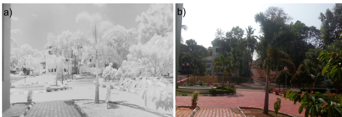
Figure 4.22. Photographs taken with a) normal camera and b) camera equipped with the VONIRT filter (NIR source: sunlight).
