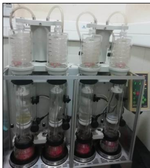
Fig.2.2. Buchi B-811 soxhlet extraction system
