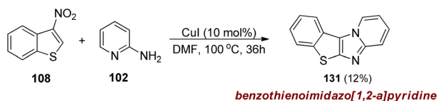
Scheme 32 Synthesis of benzothiophene-fused imidazo[1,2- a ]pyridines from electrophilic 3-nitrobenzothiophene.
