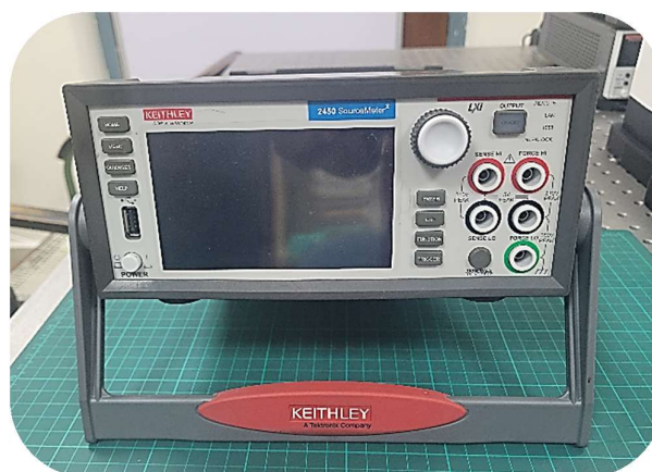
Figure 1.10: Photograph of Keithley 2450 Source measuring unit
