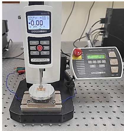
Figure 1.12: Mark-10 motorised force impactor with digital force gauge
