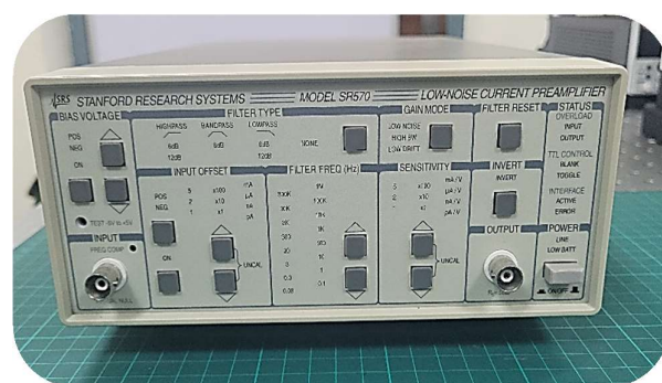
Figure 1.11: Low noise current preamplifier (SR570)
