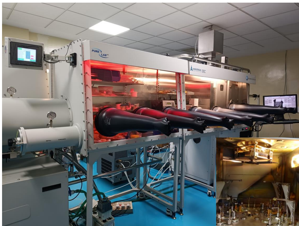
Figure A.3. Glovebox integrated thermal evaporation system (inset shows the internal view of the evaporation chamber).
