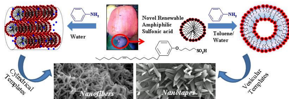
Figure 4.3. Schematic representation of the approach for synthesis of polyaniline nanofibers and nanotapes by emulsion and dispersion routes respectively.
