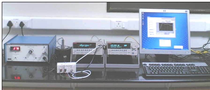
Figure 2.24. Photograph of Keithley Four Probe set up.
