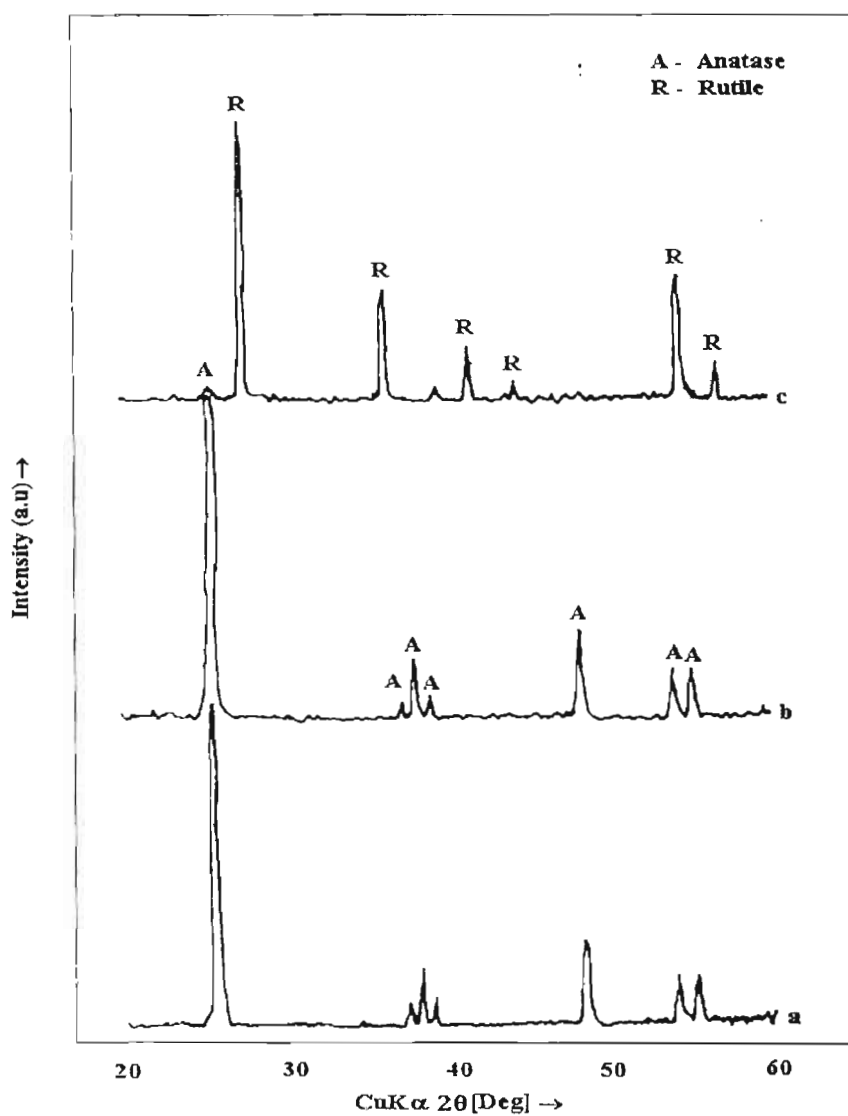
Figure 3.3: XRD patterns of undoped \text{TiO}_2 heated at different temperatures. (a) 800^\circ\text{C} (b) 900^\circ\text{C} (c) 1000^\circ\text{C}
