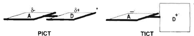
Figure 1.2. Schematic representation of geometries for PICT and TICT states for donor (D) acceptor (A) substituted conjugated systems. Adapted from reference [Yang et al. 2006].
