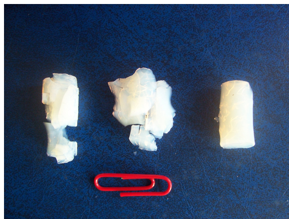
Fig. 4.2.2. Photograph of TMCS modified aerogel
