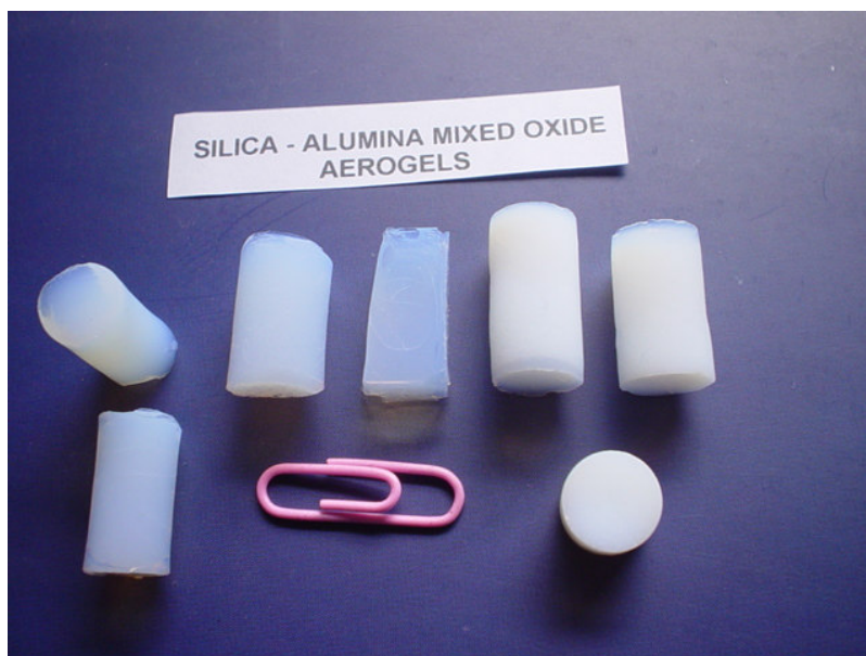
Fig. 2.2.2. Photograph of silica-alumina mixed oxide aerogels
