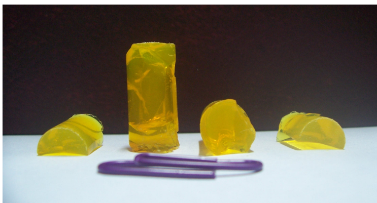
Fig. 4.1. 15. Photograph of Silica-Titania aerogel prepared by impregnation
