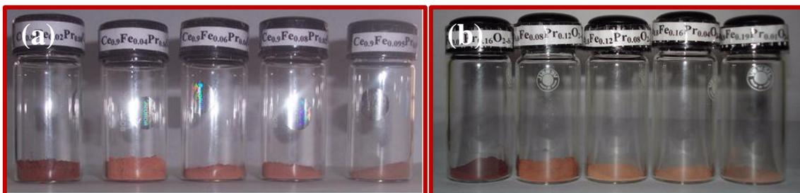
**Fig. 2.14.** Photographs of (a)  $Ce_{0.9}Fe_xPr_{0.1-x}O_{2-\delta}$  ( $x = 0.02, 0.04, 0.06, 0.08$  and  $0.095$ ) and (b)  $Ce_{0.8}Fe_xPr_{0.2-x}O_{2-\delta}$  ( $x = 0.04, 0.08, 0.12, 0.16$  and  $0.19$ ) pigments.
