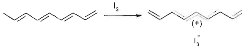
Figure 1.11. Doping of polyacetylene with iodine.
