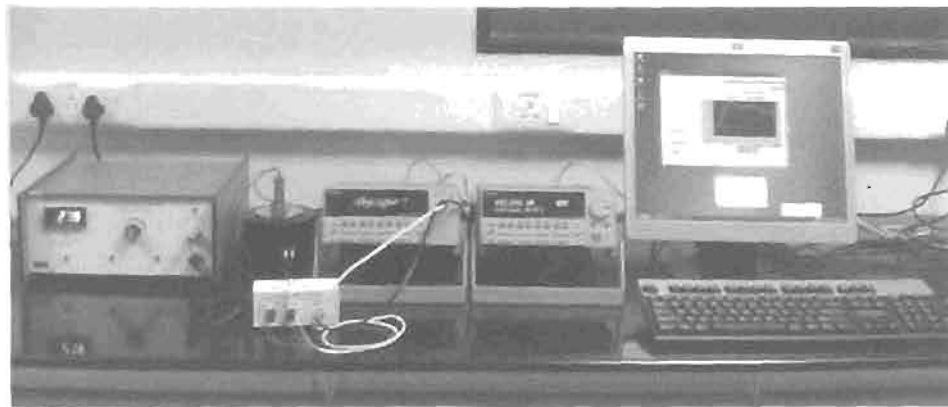
Figure 4.12. Photograph of Keithley Four Probe set up.
