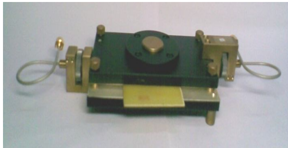
Fig. 2.3 Photograph of QWED split post dielectric resonator
