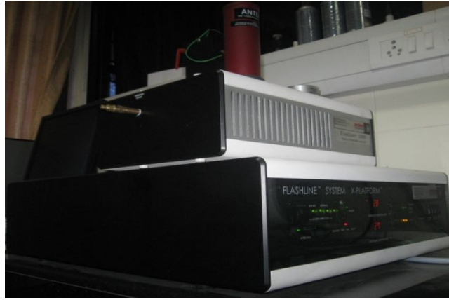
Fig. 2.5 Photograph of Flash Line™ 2000 thermal properties analyzer
