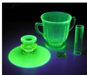
Figure 1.22: Green coloration of glasses provided by uranium
