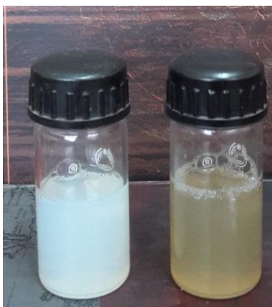
Fig. 4.12 Visual change in the colour of BLNP dispersion to yellowish, after the addition of KMnO 4 , indicating the oxidation of Ce 3+ to Ce 4+ .
