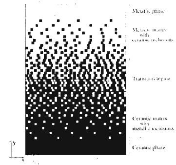
Fig. 2: Schematic Illustration of an FGM with continuously graded microstructure.
