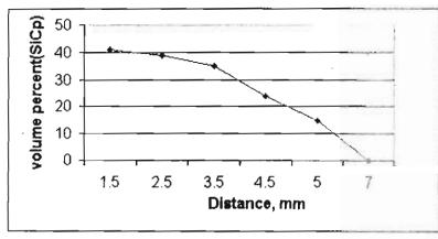
Fig. 8: SiC Particle distribution in Al (6061)-SiC FGM10.
