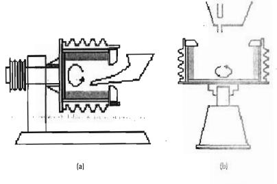
Fig. 1: Schematic sketch of (a) Horizontal and (b) Vertical Centrifugal Casting.
