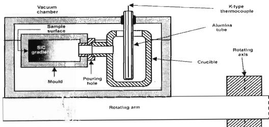
Fig. 3: Schematic setup of the Centrifugal Casting for producing FGM Using Vacuum Chamber⁵.
