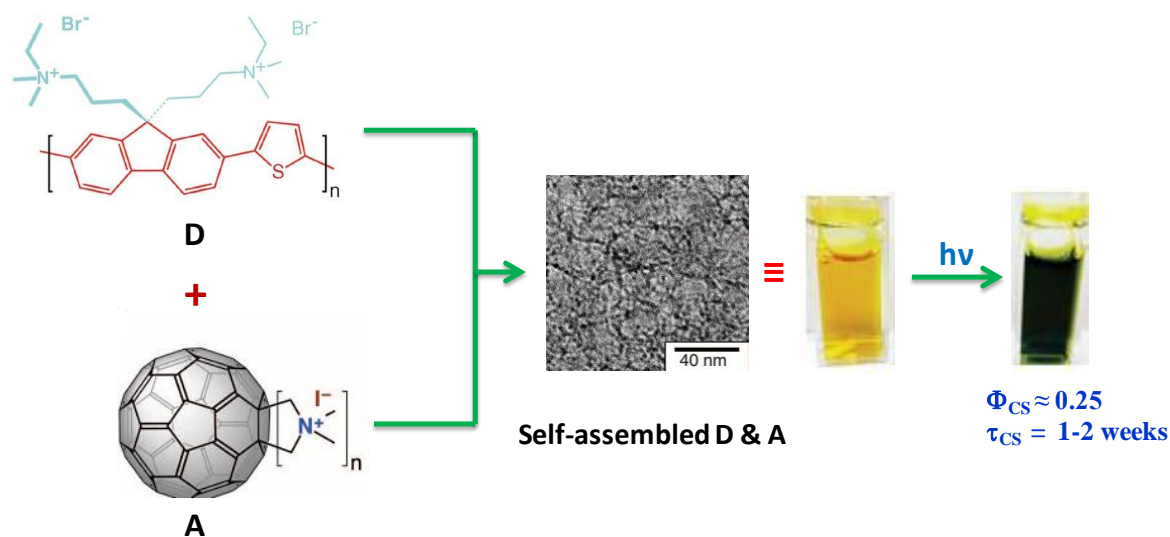
Figure 4.4. Schematic of the self-assembly of D and A leading to the formation of long-lived CS state.
