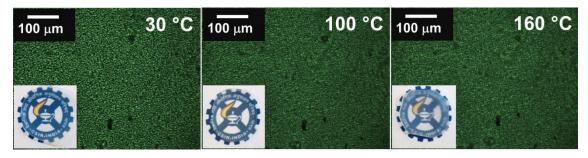
**Figure 2.11.** POM images of PLLA films crystallized in acetone/water mixture measured at (a) 30 °C, (b) 100 °C, and (c) 160 °C. Photographs showing the transparency of PLLA films at different temperatures are shown in the inset.
