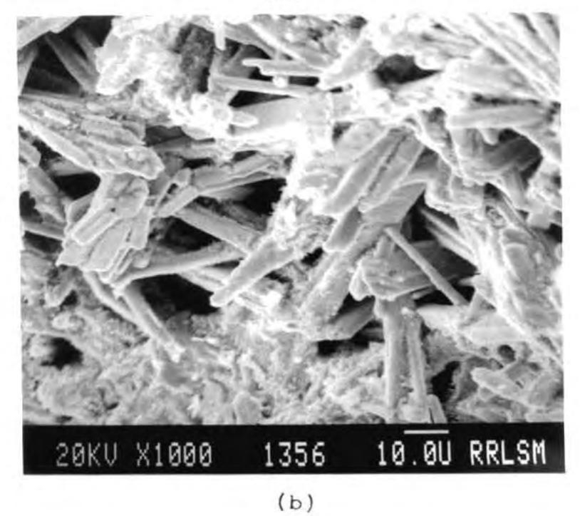
Fig. VI.2 SEM picture of the morphology of the YBCO derived through (a) Citrate and (b) Flash combustion gel decomposition
