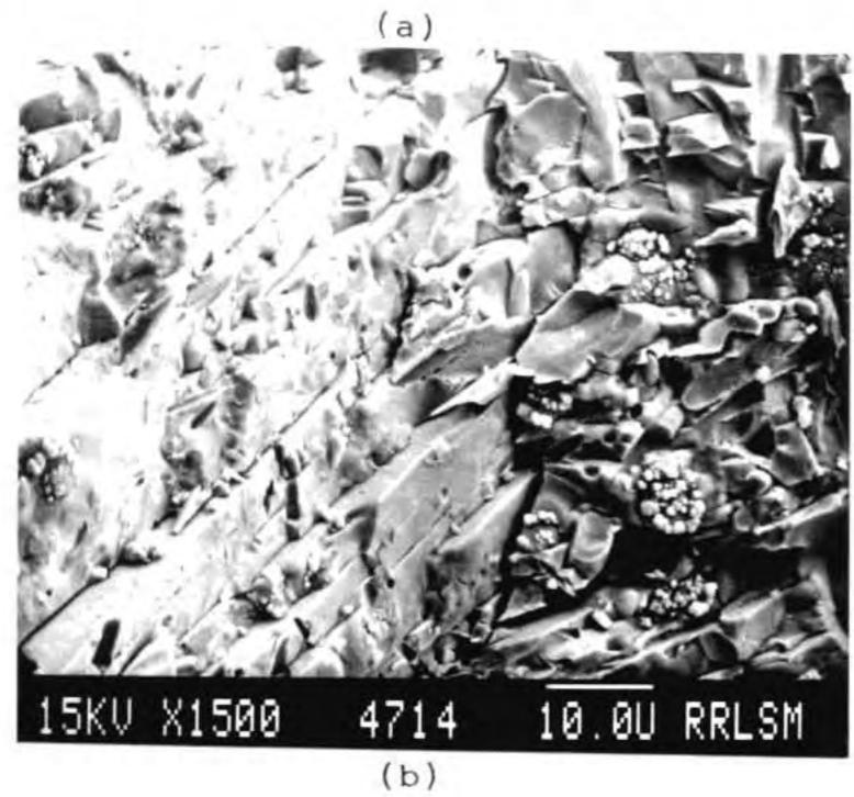
Fig. V.12 SEM pictures of fractured zone refined samples showing bulk oriented YBCO grains
