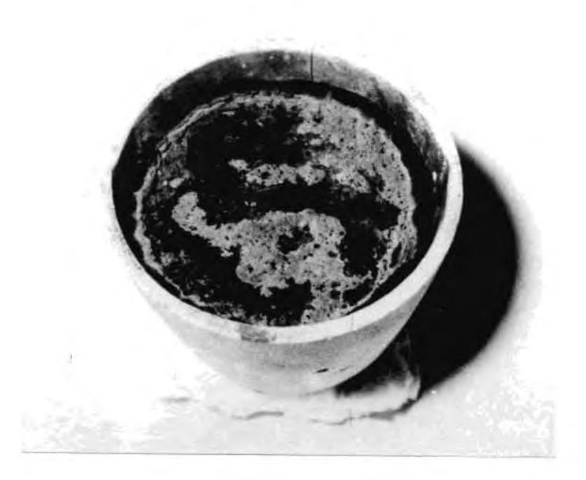
Fig. V.2(b) Precursor powder inside the crucible
