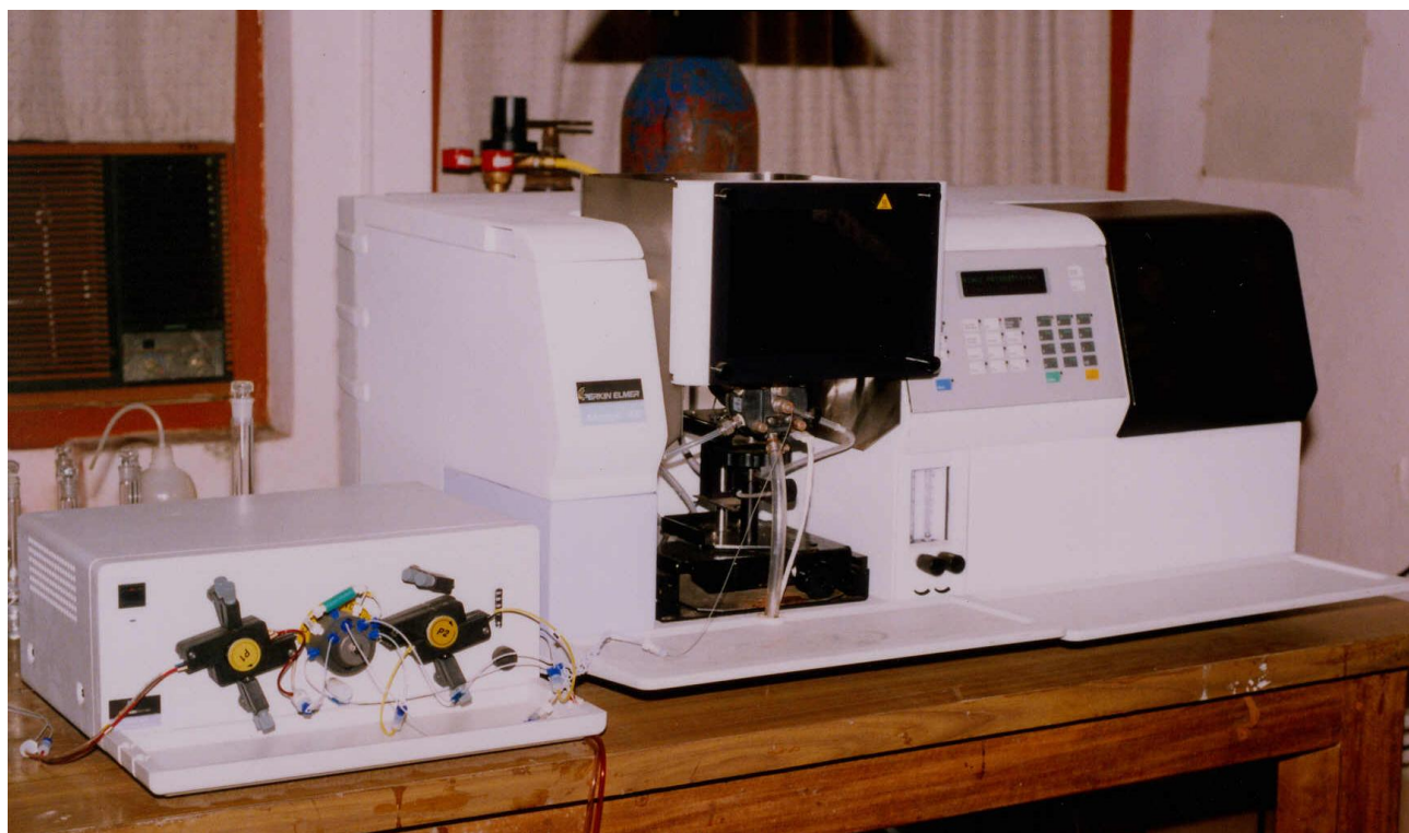
Fig.5.7: Flow Injection-FAAS for online preconcentration & Determination
