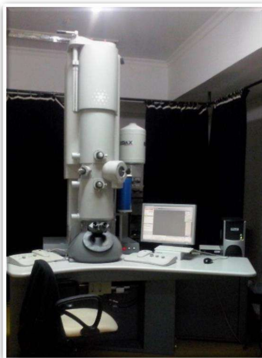
Figure 3.10. FEI Tecnai G230S Twin 300 kV TEM facility at NIIST, Trivandrum.
