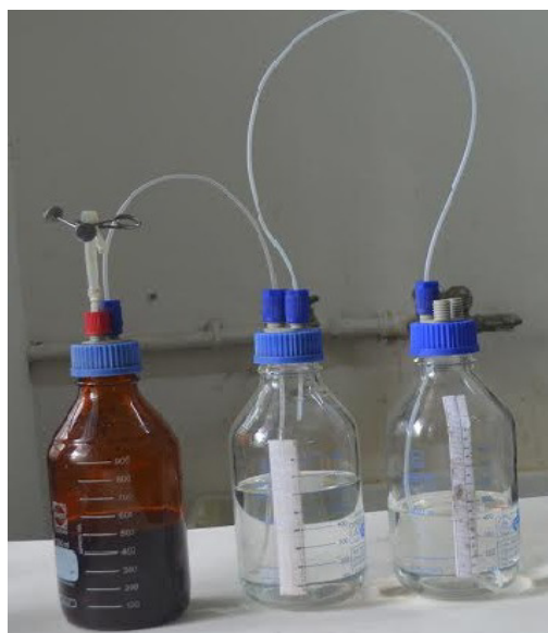
Figure 5.1: Batch biomethanation set up for digestion of water hyacinth and Pistia sp., biomass
