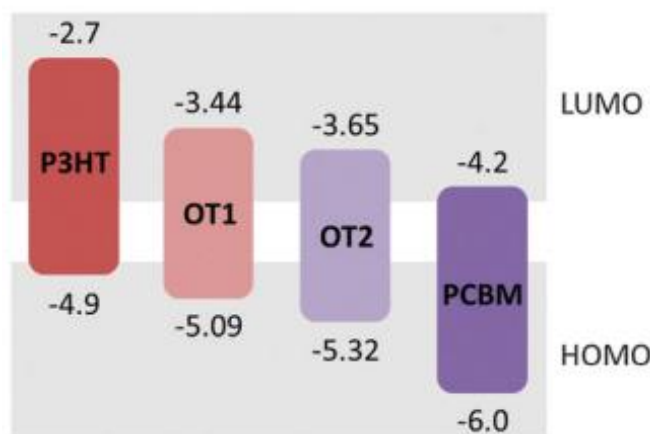
Figure 2.9. Scheme showing the comparison of the HOMO–LUMO levels of the oligomers with that of P3HT and PCBM.
