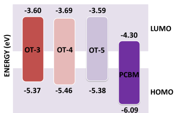
Figure 3.9. HOMO-LUMO energy levels of the oligomers compared to that of PC 71 BM.
