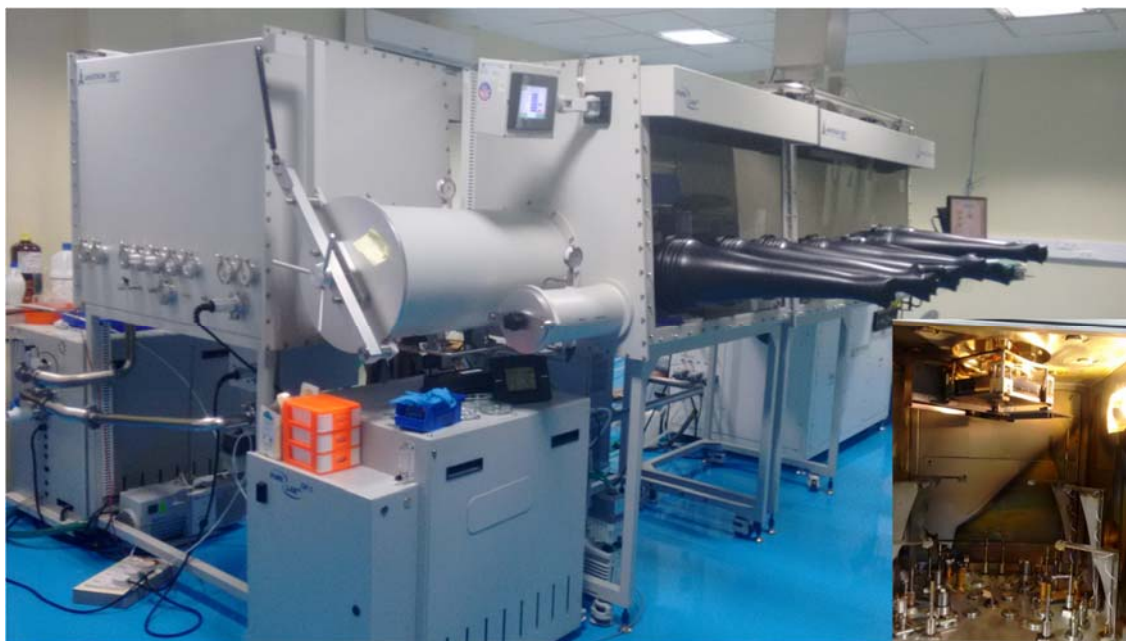
Figure A.1 Glovebox integrated evaporation system; inset shows the internal view of the evaporation chamber
